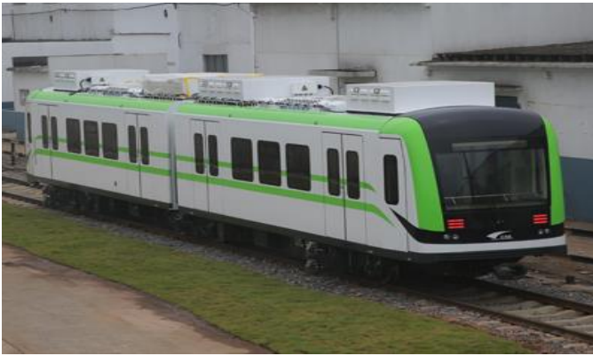
Figure 5: Subway CSR Zhuzhou Electric Locomotive with supercapacitors to power the electric motors.
